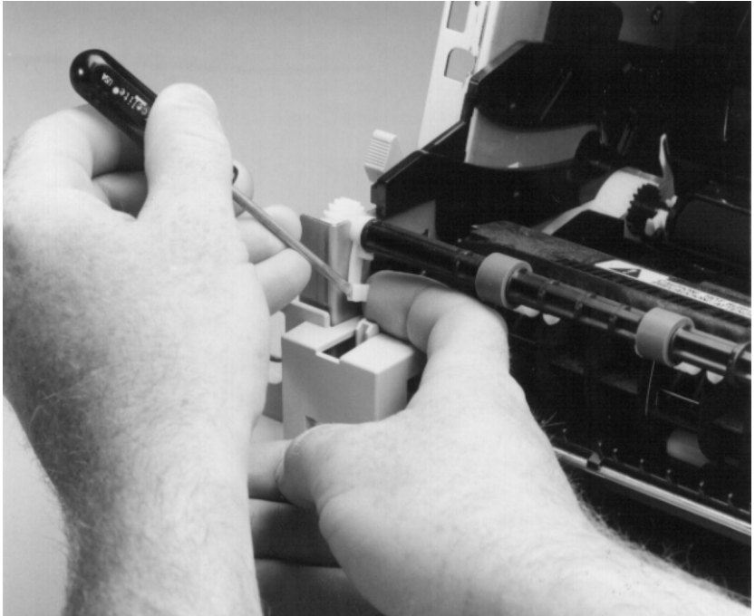
Figure 39. Exit roller removal
